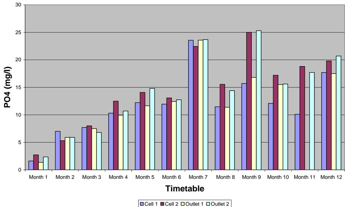
Fig. 15. Data showing phosphate content for both cells during the monitoring period.
