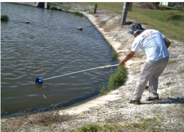
Fig. 10. Water samples were collected in order to establish baseline levels of BOD, salinity, nitrates, orthophosphates, and turbidity.
