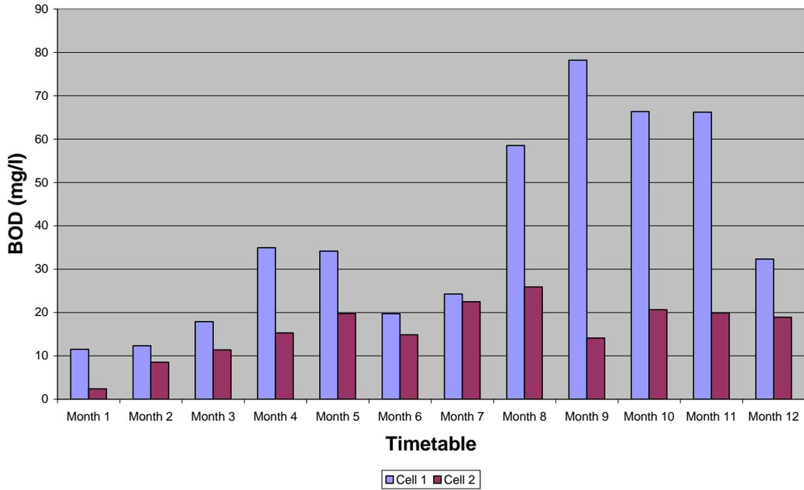
Fig. 12. Data showing BOD for both cells during the monitoring period.
