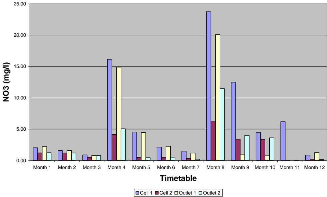
Fig. 14. Data showing nitrate content for both cells during the monitoring period.
