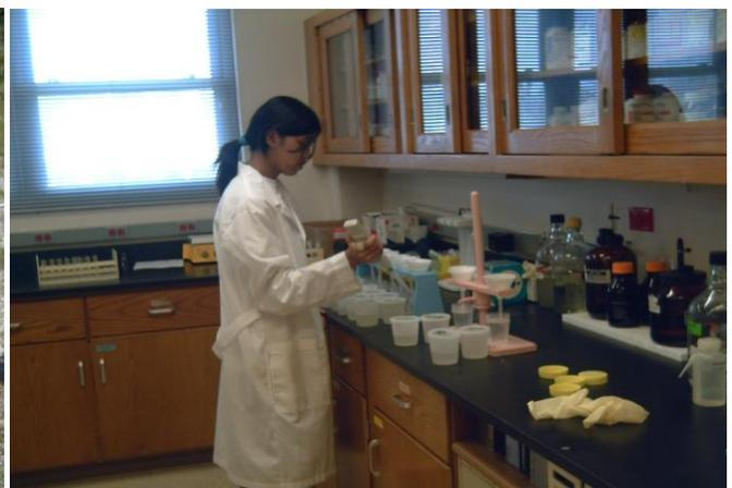
Fig. 11. Student intern filtering water samples for nutrient analysis at the UOG Soil Lab.
