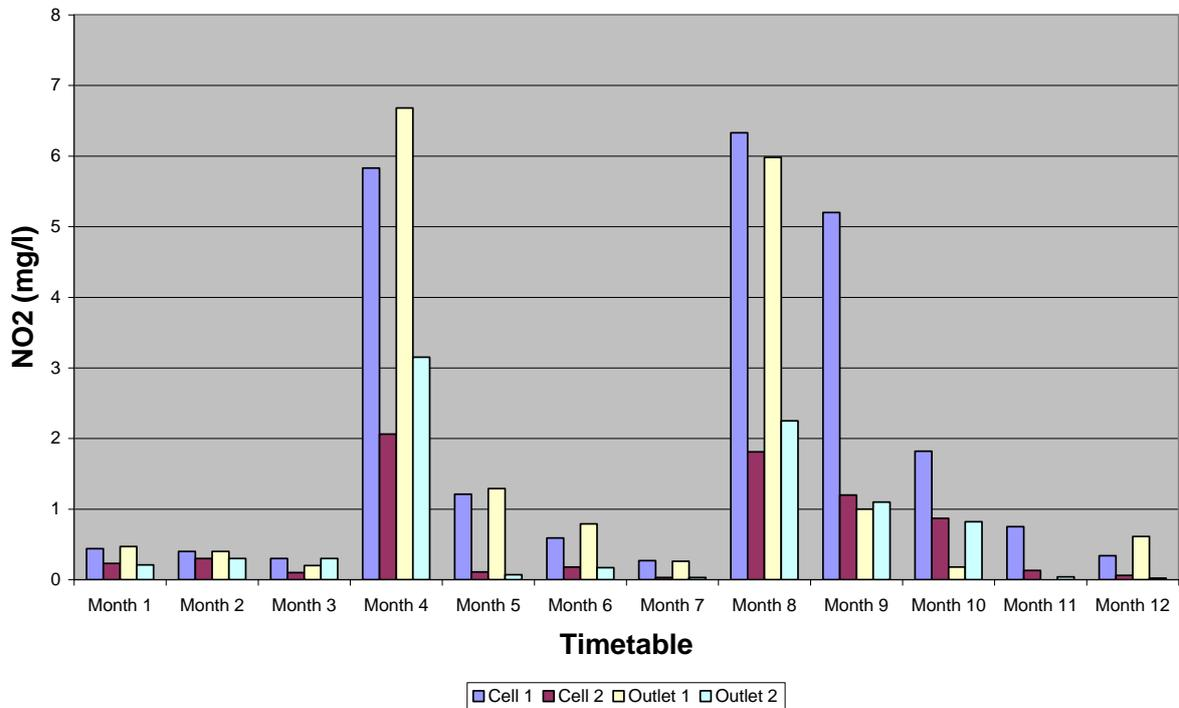
Fig. 13. Data showing nitrite content for both cells during the monitoring period.
